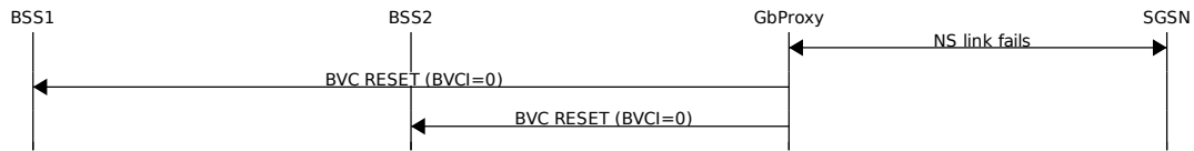
Figure 4: SGSN connection fails
