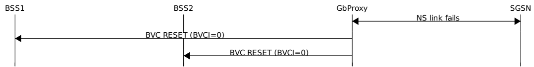
Figure 4: SGSN connection fails
