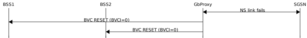
Figure 4: SGSN connection fails
